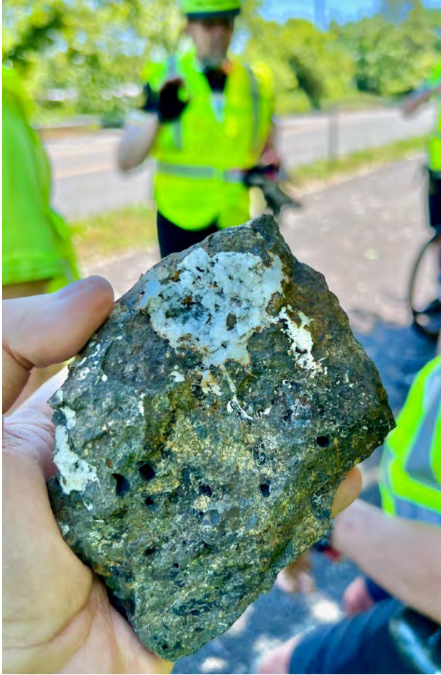
The Waverley Basalt contains zeolites formed by hydrothermal fluids circulating through the original rock. Photo by Paul Edison-Lahm.
