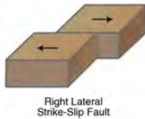
The main sense of slip across a strike-slip fault is horizontal. To recognize a right-lateral strike-slip fault, the block on the opposite side of the fault from an observer has moved to the right.
